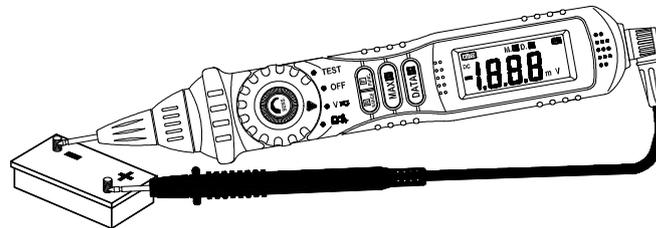
4.7.5 Connect the probe tip of the meter and probe tip of the test lead (or test clip) across the power source or be loaded on the two sides under measurement.
